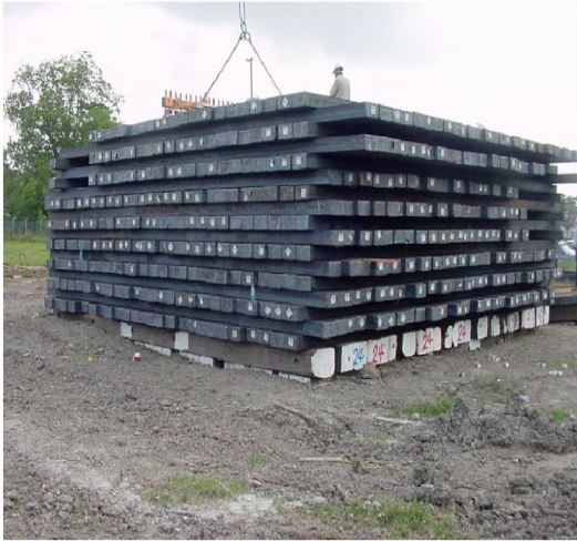
Photograph 2. One of three test cells, each with a different replacement ratio, fully loaded with 1 million kilograms of steel ( 177 \text{ kN/m}^2 ) (Cali et al., 2005).
